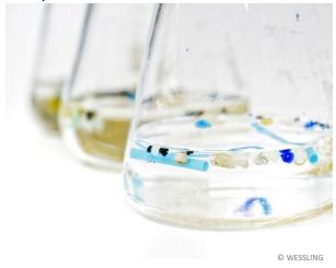
MIR-spectroscopy is currently used for the detection and analytics of microplastic in water. The absorption of light is used in mid infrared by plastic particles to identify and classify small particles – a very complex method that the partners of the SIM-QPla project want to revolutionize.
